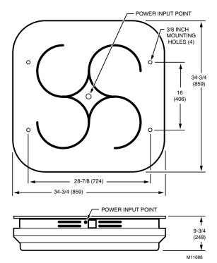
Fig 1. F115 dimensions in in. (mm).
